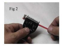
Before sending this blade off to the sharpener clean any hair that could be trapped under the cutter. Its simple and could save you the expense of sharpening or buying a new blade.
