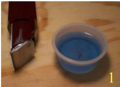
1. Get your H-42 dip and your blade. Clean as much of the hair from around the spring and teeth with your toothbrush. (See our tips on cleaning blades) Attach the blade to your clipper as shown. You are now ready to clean the blade using the H-42 as a dip.
