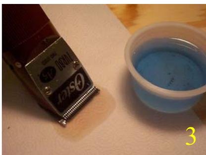
3. Have a paper towel handy and with the clippers off, pull the blade from the H-42 and grab it with the towel to prevent dripping all over. Continue to wipe the blade until you are satisfied its dry enough. You can even take the blade off the clipper and wipe both sides dry. Be sure to wipe the end of the clipper dry as well. Never hold the clipper straight up because the H-42 may get sucked inside. The blade is now clean, lubed, and ready to use all by using one step cleaning.
