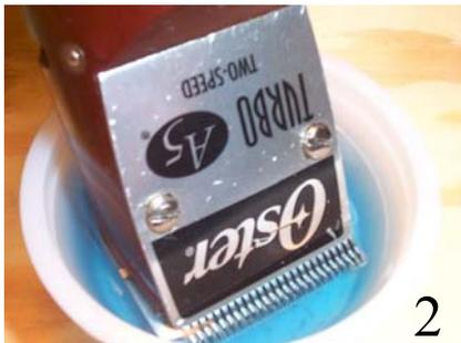
2. Hold the clipper with both hands for steadiness and just put the blade into the H-42 far enough to cover the teeth. Now turn the clipper on. Immediately the motor will start to gain rpm's and there will be black stuff being washed into the dip, you can see it if you look. Hold it there until you feel its clean enough then turn clipper off before pulling it out.
